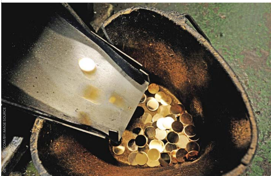
➤ Below: Pure gold sheets are stamped into blank disks, to be minted into Krugerrands.
