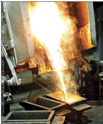
➤ Above and below left and right: A gold pour is performed at the gold plant of a Western Australian gold mine. The finished bar is then transported to a gold refinery for processing to 99.999 percent purity.
