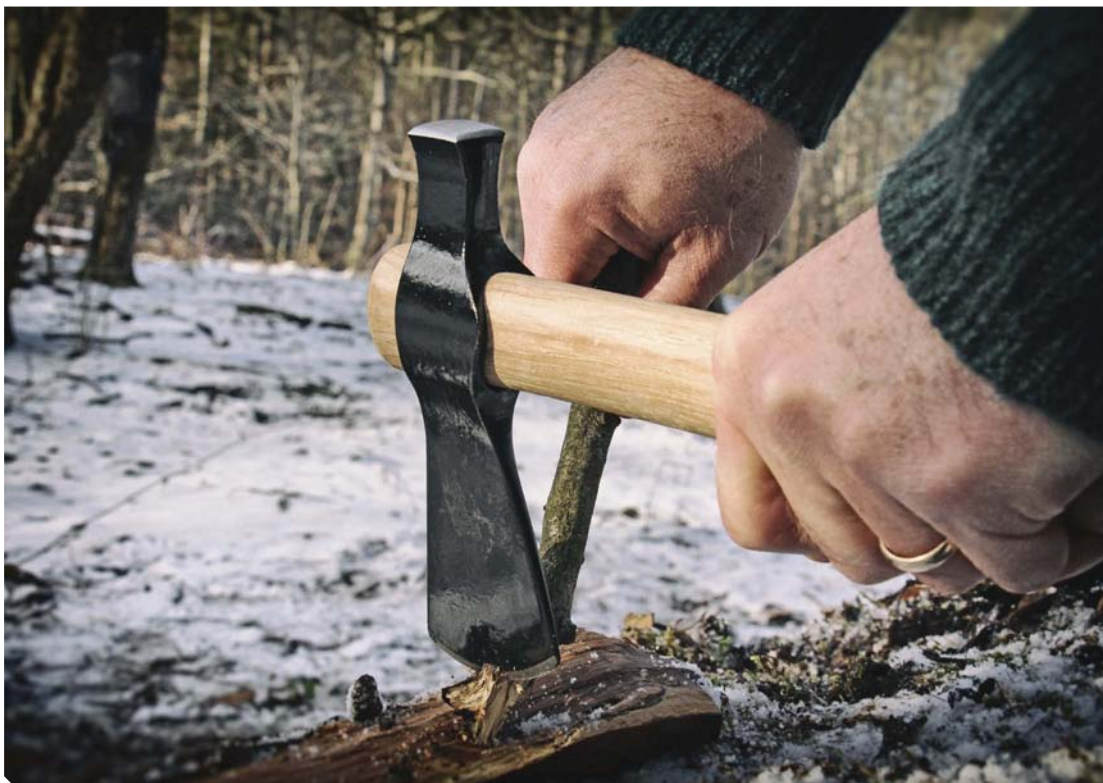
◀ For detail work and making more-precise cuts, choking up on the handle gives you greater control, as shown with this Cold Steel Trail Hawk.
