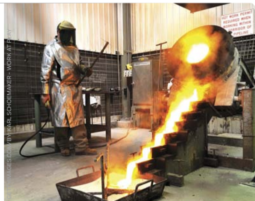
➤ Above and below left and right: A gold pour is performed at the gold plant of a Western Australian gold mine. The finished bar is then transported to a gold refinery for processing to 99.999 percent purity.
