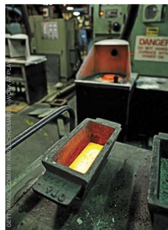
➤ Above and below left and right: A gold pour is performed at the gold plant of a Western Australian gold mine. The finished bar is then transported to a gold refinery for processing to 99.999 percent purity.
